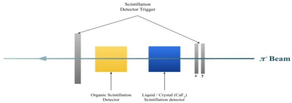
Figure 2: Experimental Setup diagram for T9 laboratory using a beam of negative pions at a range of 2-6 GeV.
