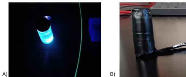
Figure 7: A) Kidneywood pigment emission using a UV-lamp of 365 nm. B) the detector is already assembled.
