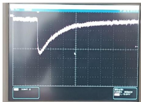
Figure 8: Signal obtained by the Kidneywood liquid pigment scintillator, this signal proved to be 18 mV.
