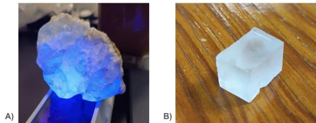
Figure 3: A) Raw Fluorite crystal obtained in Peña de Bernal, Mexico. B) Raw fluorite was cut into an approximately 1cm<sup>3</sup> sample.
