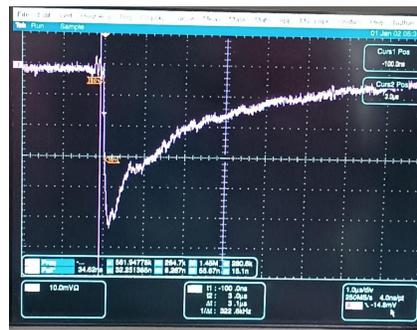
Figure 4: Output voltage signal obtained by a CaF<sub>2</sub> detector. The signal was 50 mV.
