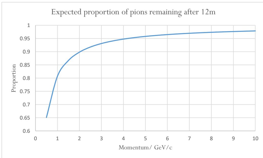
This graph shows our theoretical predictions for the number of decaying particles having travelled 12 metres through the experimental area. It indicates that there should be a measurable difference in the number of particles at different momenta.
