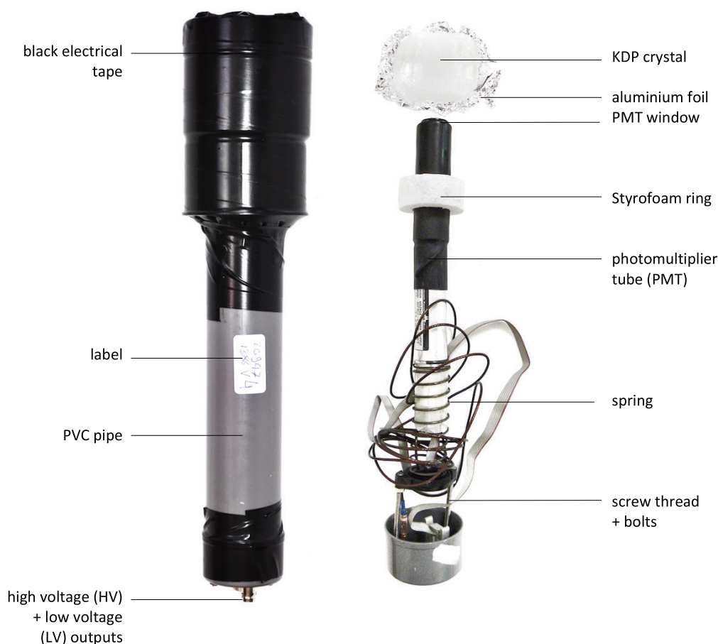
Figure 3. Complete setup of the outside (left) and inside (right) of an individual module of our calorimeter.
