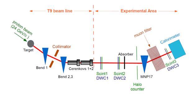
The incoming 24 GeV/c primary proton beam from the PS impinges on a target. The collisions of the protons with the target nuclei provide a variety of particles. The T9 secondary beam line is set up to select the particles of various momenta, between 0.5 and 10 GeV/c. This selection is based on the deflection in the bending magnets (Bends 1-3) and the collimator, and is further refined by quadrupole lenses.
